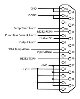
Pins 1, 2, 3, 4, 12, 24 - +5 VDC. It is important to have all pins connected for proper operation.
