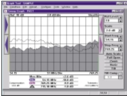
▲ The detailed forward or reverse sweep graph offers user-adjustable markers, scale, reference level, and tilt. Users can clearly distinguish the difference between previous and current sweep measurements for easy comparison on the PC StealthWare display.
