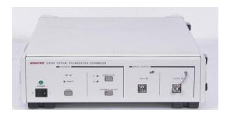
The Q8163 is a optical polarization scrambler which has a function to change the state of output light polarization with using a polarization element of optical fiber type. The state of output light polarization can be changed continuously by driving 3 polarization elements of optical fiber type. Therefore, all the states of polarized light (all the points on the Poincare sphere) can be output.
