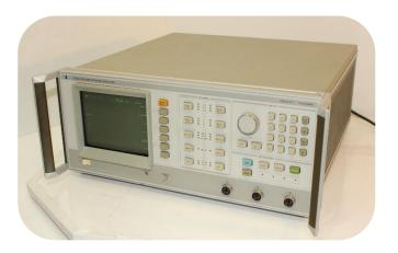
Measure insertion loss and gain, return loss, and absolute power quickly and accurately with the 8756A scalar network analyzer. These scalar measurements can be performed over a broad 10MHz to 60GHz frequency range.
