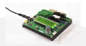
ULDC is a fully integrated laser diode controller with precise current and temperature setting. With a Zero Insertion Force (ZIF) adaptor, ULDC can be used with all 14 pin laser diodes. It also features ~2MHz direct modulation with external board
