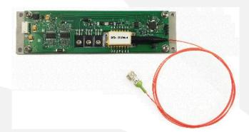
DFB-1550H-PM can be ordered as DFB- PM-M, which allows DFB laser's operating temperature and output power precisely controlled to ensure constant wavelength and power stability. It can be used for module level integration system.
