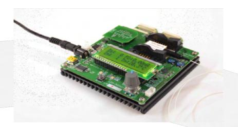
ULDC is a fully integrated laser diode controller with precise current and temperature setting. With a Zero Insertion Force (ZIF) adaptor, ULDC can be used with all 14 pin laser diodes.
