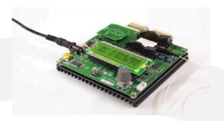
ULDC is a fully integrated laser diode controller with precise current and temperature setting. With a Zero Insertion Force (ZIF) adaptor, ULDC can be used with all 14 pin laser diodes.
