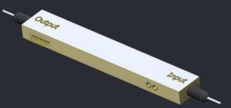
Optilab's QPSK-1550-12-SQ, Quadrature Phase Shift Keying (QPSK) modulator, is a dual parallel structure of two Mach-Zehnder modulators embedded in a Mach- Zehnder super-structure. Each internal modulator is designed to support 12 Gb/s signals.
