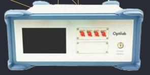
Optilab DFB-4-B is a Distributed Feedback (DFB) laser source in a benchtop unit designed for general laboratory applications. The DFB laser's operating temperature and drive current are precisely monitored by a microcontroller to ensure constant output power and emission wavelength stability. Using its intuitive front panel or an optional USB interface, the user can control the DFB output power level by adjusting the laser drive current and emission wavelength via TEC.
