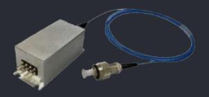
Optilab's LD-785-40-PM-CM & LD-850-70-PM-CM is a 785 nm & 850 nm pigtailed laser module, with an 8pin package. This high-efficiency and high stability product is featured in a TEC cooler and internal photodiode. The 785 has a 40 mW output power with the 850 version having a 70 mW output power. Both devices have 5  $\mu$ m PM fiber and can be used in medical laser treatment and biotechnology. 785 & 850 nm wavelengths.
