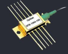
Optilab DFB-1064-PM-100-CW is a Distributed Feedback (DFB) Laser with 100 mW output power designed for Continuous Wave (CW) operation. It is mostly utilized in combination with an external optical modulator, such as a Mach-Zehnder Interferometer (MZI) modulator.
