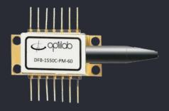
Optilab's DFB-1550C-PM-60 is a single frequency laser coupled with Polarization Maintaining fiber. Built with Distributed Feedback Grating (DFB) as cavity reflector, it provides pure, single longitudinal mode, hopping free and extremely stable wavelength source. This laser diode is fabricated with Multiple Quantum Well (MQW) for excellent reliability and stability (also comes in wavelengths from 1549 ~ 1553 nm with output powers of 40, 50, 60 mW).
