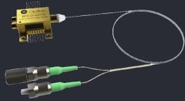
Optilab's PR-30-SQ is a linear photo receiver designed for analog applications. This compact photo receiver contains a surface coupled coplanar waveguide PIN photodiode and a linear transimpedance amplifier within a hermetically sealed 14-pin butterfly package. With an integrated variable gain amplifier (VGA).
