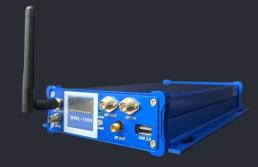
Optilab's SWL-1550-MC is a laser source module unit provides fast continuous wavelength sweeping, driven by an electrical ramp voltage input, and contains a fast tunable laser source with control electronics (available in rackmount housing and in 1540, 1558, and 1566 nm wavelengths).
