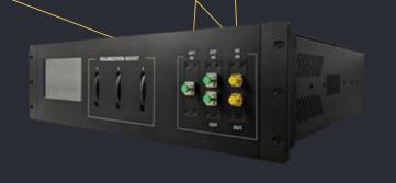
Optilab's LLA-1310/1550-R is a laser linewidth analyzer based on the delayed self-heterodyne interferometric technique. It consists of a high-performance LiNbO3 phase modulator as the frequency shifter in the delayed self-heterodyne interferometer.
